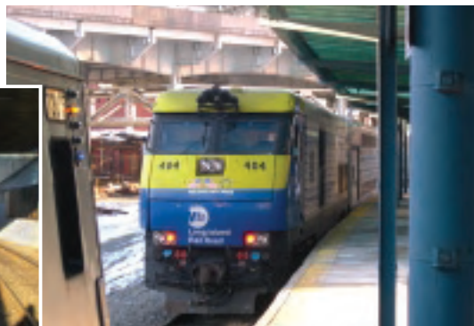
When pulled by a locomotive (left), pollution from the engine invades the coaches behind. When the train is pushed, the pollution plume trails behind leaving in-coach levels low (right).
