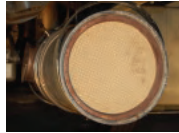
Above: Honeycomb particle trap from DPF on box truck.
