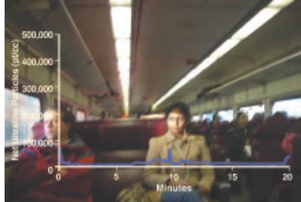
In-coach levels of ultrafine diesel particles in this test were 10-100 times higher in coaches being pulled by a locomotive (left) than in coaches being pushed (right).
