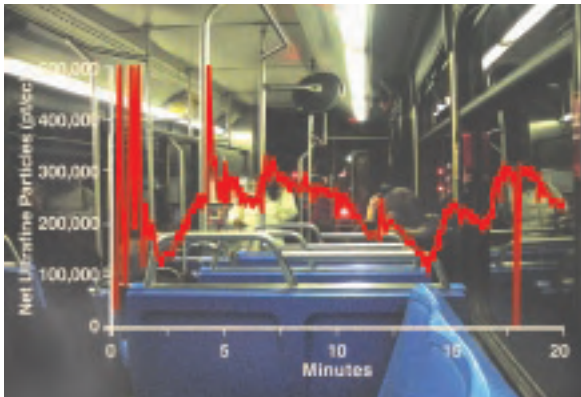
CATF researchers measured high ultrafine particle levels on a conventional transit bus in Boston (left), while levels on a bus retrofitted with a particle filter were barely detectable (right).
