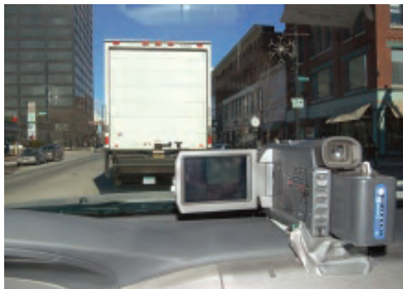
A dashboard-mounted digital video camera inside the chase car allowed researchers to film the driver's-eye-view behind the diesel vehicles while monitoring instruments recorded pollution levels inside the car. To view videos, go to www.catf.us/goto/noescape/
