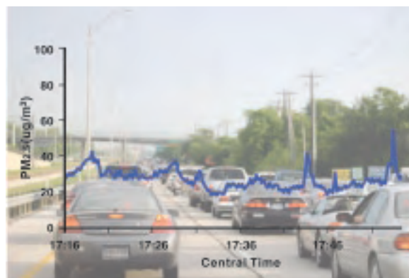
In-cabin fine particle exposures are much higher for commuters along routes with diesel trucks. The MOPAC highway (right) a no-truck alternative to I-35 (left) in Austin, Texas, had lower diesel pollution levels.
