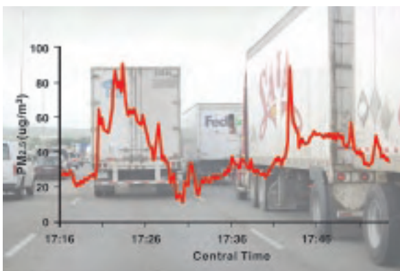
In-cabin fine particle exposures are much higher for commuters along routes with diesel trucks. The MOPAC highway (right) a no-truck alternative to I-35 (left) in Austin, Texas, had lower diesel pollution levels.
