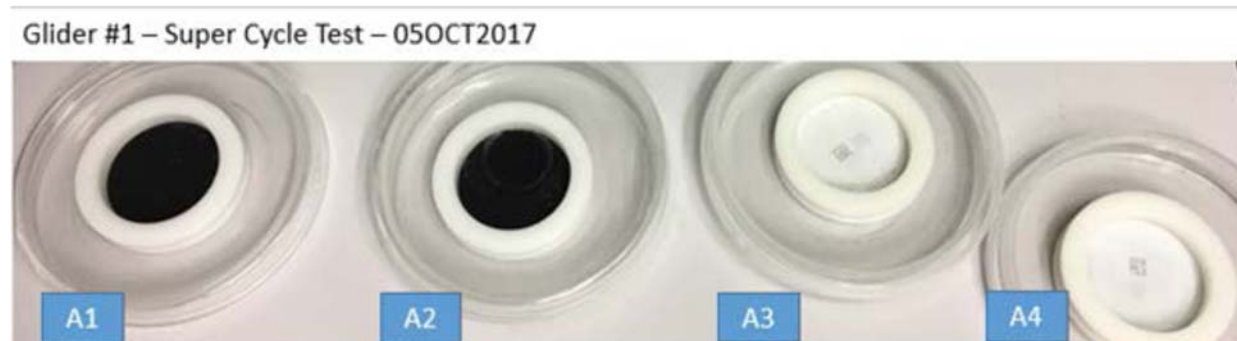
Figure 9: PM Filters from Glider #1 testing over the Super Cycle Test
